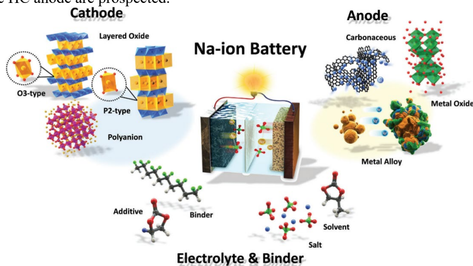
Figure 1 Illustration of a Na-ion Battery System [7]
